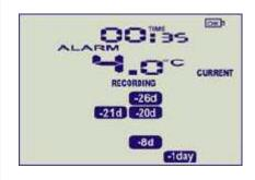
If a reading outside the pre-set "Alarm" limits is recorded at any time, a "day alarm indicator" appears on the display. A visual alarm trigger is displayed if one or more of the configured alarm trigger conditions have been met. An alarm trigger condition can be a single reading above the upper or below the lower threshold values, a set of consecutive violating readings or an accumulation of violation readings encountered.
