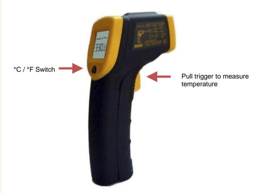
The display is simple but has all of the controls that professional users need. The laser beam can be triggered on and off for safety reasons (required in some applications).
